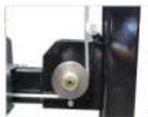
For safety mechanism protect quickly declined cause by wire rope breakage.
