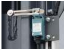
Upper limit switch
