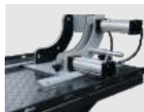
Pneumatic fixed front wheel clamp device
