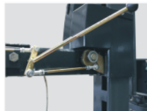
Manual safety bar for release.
