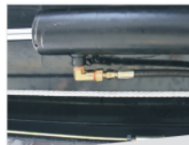
Oil cylinder with explosion-proof valve.
