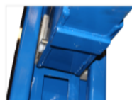
Nylon slide board for limit insurance piece.
