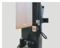
Down limit and oil-mist separator.
