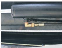
Oil cylinder with explosion-proof valve.
