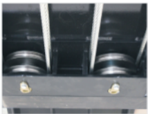
Cable and pulley under main platform.
