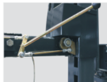
Manual safety bar for release.
