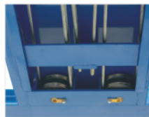
cable and pulley under main runway.
