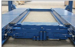
Optional pneumatic or electric rolling jack, Optional rouing jaek. Capacity 3.2T(7000 pounds).
